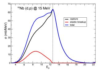
elastic breakup and capture cross sections as a function of the proton energy. The Koning–Delaroche global optical potential has been used as the  $U_{An}$  interaction (Koning and Delaroche, Nucl. Phys. A **713** (2003) 231).
